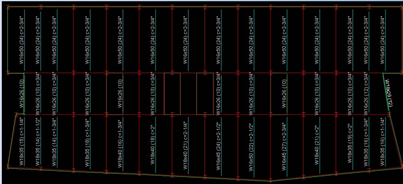
Typical floor layout of cambered beams
